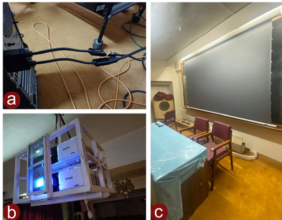
Fig. 1 Hardware of AnaVu . a Showing the dual output through HDMI from the CPU used for the AnaVu software system. b Showing the two projectors stacked one above the other, mounted within a projector cage. Polarization filters are also seen in front of the projectors. c Showing the silver screen used for the stereoscopic projection
