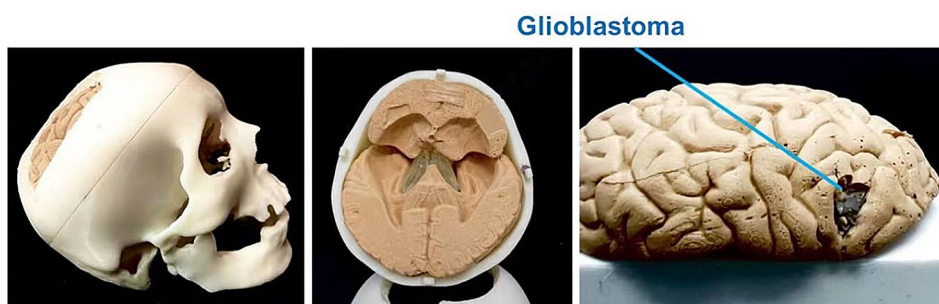
Fig. 1 The PLB simulator. The different structures are marked in different colors: skull (white), glioblastoma (grey), and lobe (beige)
