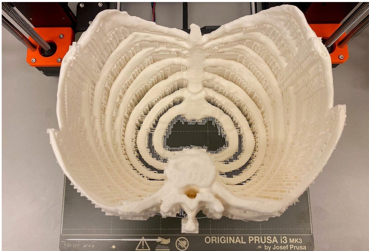
Fig. 3 3D-printed model of the bony thorax on the print bed
