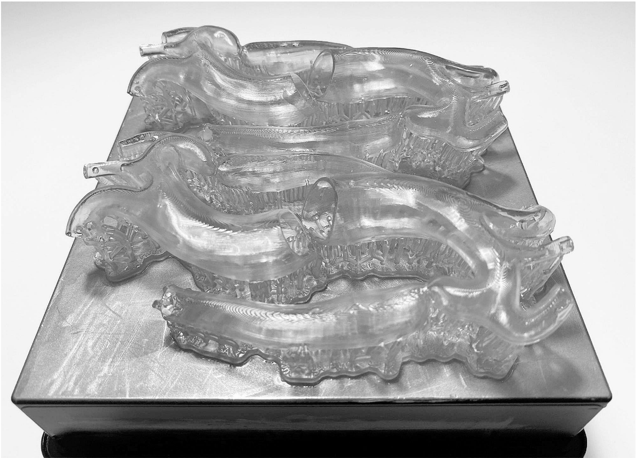
Fig. 2 3D-printed models of the CoA manufactured from Elastic 50 A resin
